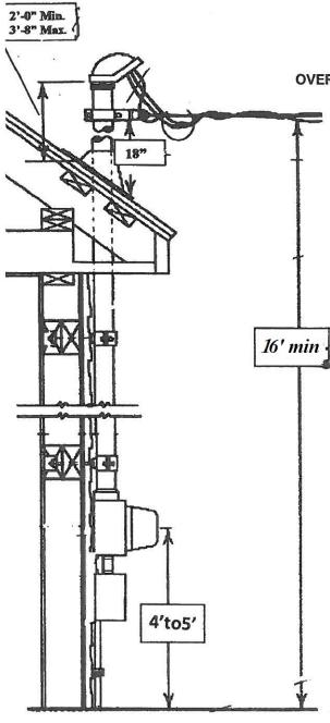
OVERHEAD SERVICE TO A PERM WEATHERHEAD ABOVE ROOFLINE
