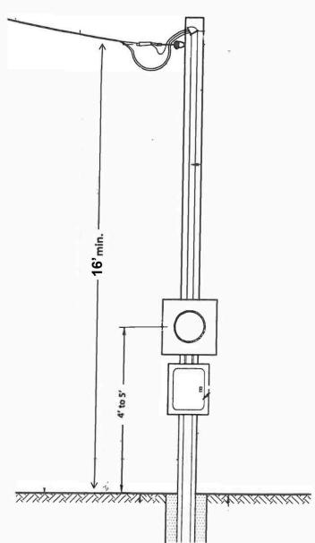
Meter loop pole shall be provided by, installed, and maintained by the Member. The service drop will be provided by and maintained by the Coop.
