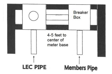
Meter loop rack shall be provided by installed and maintained by the Member. The service drop will be provided by and maintained by the Coop.
