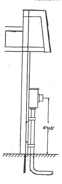
Meter base shall be provided, installed and maintained by the Member. The Coop will provide, install and maintain the service wire and conduit to the meter base.
