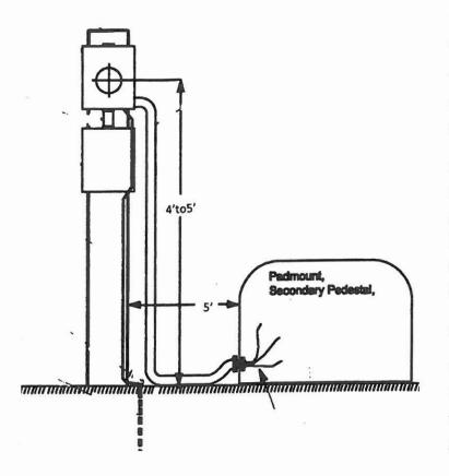
Temporary pole provided and installed by Member. Pole is to be a 4"x4" treated post or a minimum 5" treated pole set 3 ft. in the ground and braced if needed.
