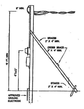
Temporary pole provided and installed by Member. Pole must provide sufficient height for the service drop provided by the Coop to meet 12 ft. minimum clearance. Pole is to be a 4" x 4" x 16 ft. unspliced braced post 3 ft in the ground or 5" minimum diameter treated pole, 4 ft in the ground or braced.
