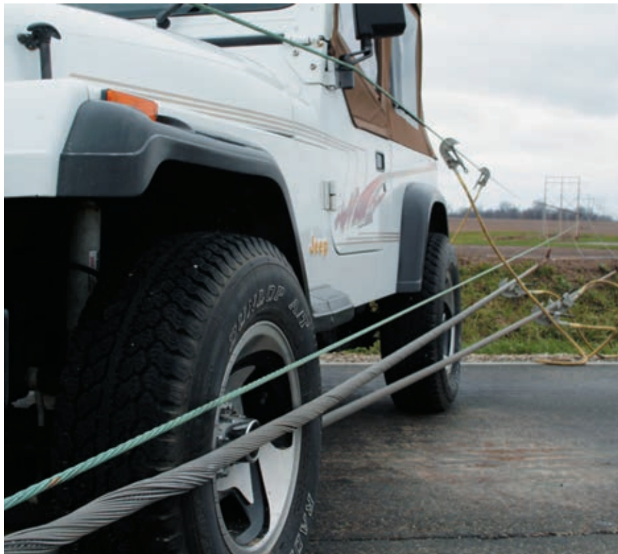
If you are in an accident involving a utility pole, stay in the car until help arrives.
